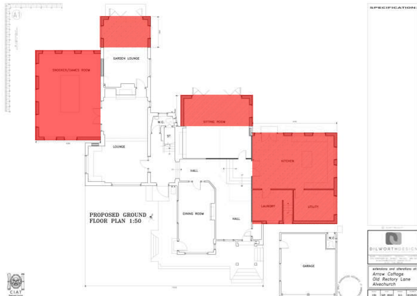
Figure 8 : Permitted Development rights Ground Floor plan, showing extensions in red (Ref.: 20/01300/CPL)
